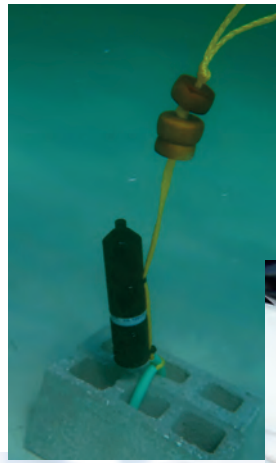
(left) Underwater acoustic receivers were deployed near the potential spawning site to "listen for" tagged bonefish. Photo by Dr. Zack Jud
